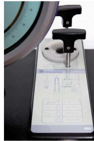
Control schematic on the CPB3800HP instrument base
