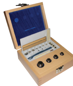
Set of fine increment masses
