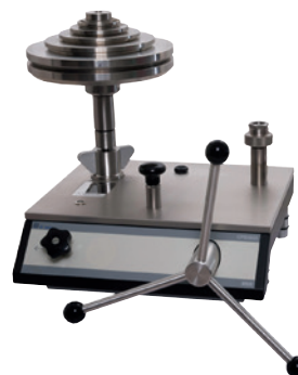
Pressure balance, model CPB5800
